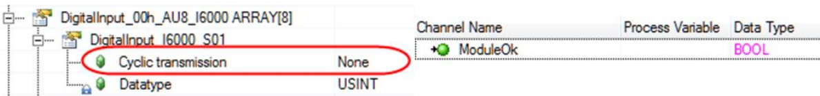
Fig. 6 Deactivation of all channels, no data points except ModuleOk
