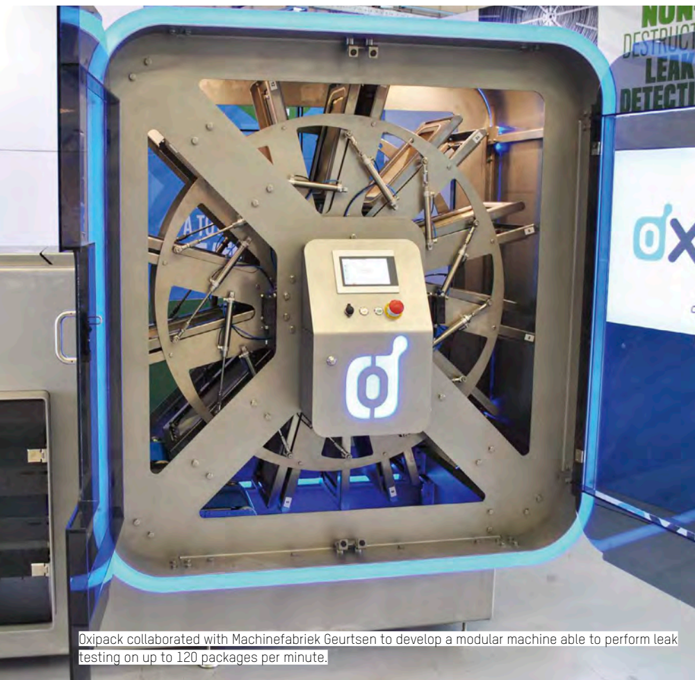
The infeed belt and rotary wheel are synchronized perfectly thanks to B&R's fully integrated motion control system.
