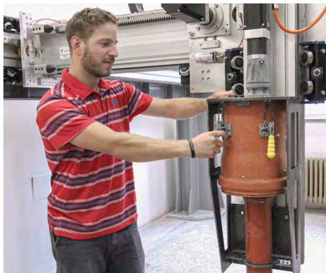
David Čítek of the Klokner Institute demonstrates the Printing Mantis print head, where a sophisticated B&R motion control solution dispenses a highly specialized concrete mix.
