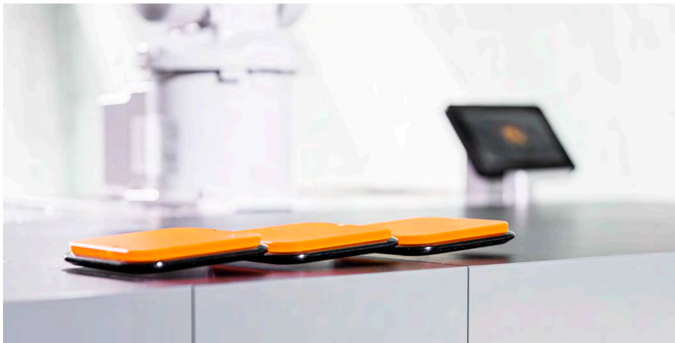
ACOPOS 6D shuttles tilt along three axes.
