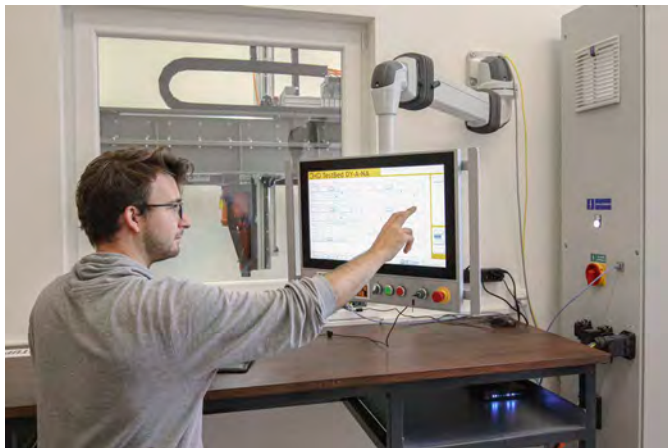
At the Klokner Institute testbed, the print head is controlled using a swing-arm HMI panel from B&R. The web-based HMI application can also be viewed on a PC, smartphone or tablet.
