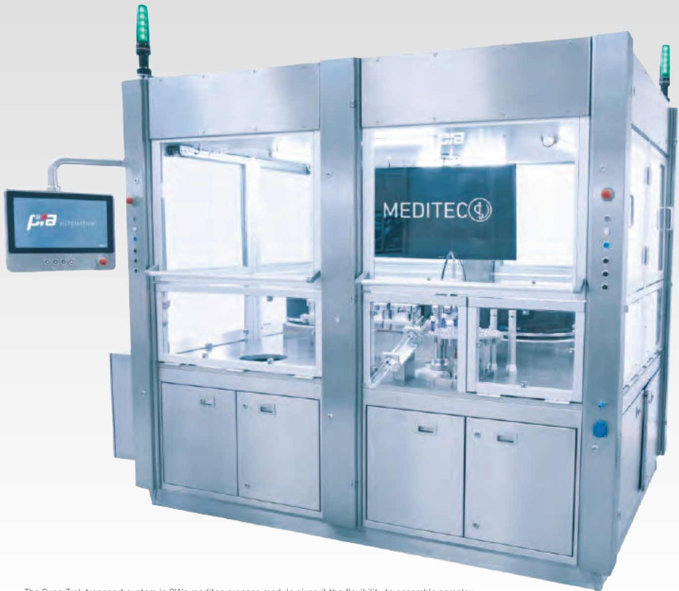
The SuperTrak transport system in PIA's meditec process module gives it the flexibility to assemble complex medical devices in large volumes – both inside and outside the cleanroom.
