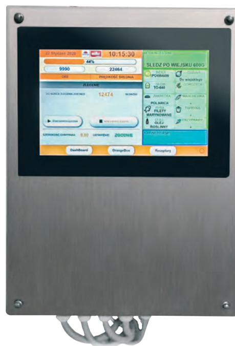
The Orange Box HMI shows a live overview of key performance data.
