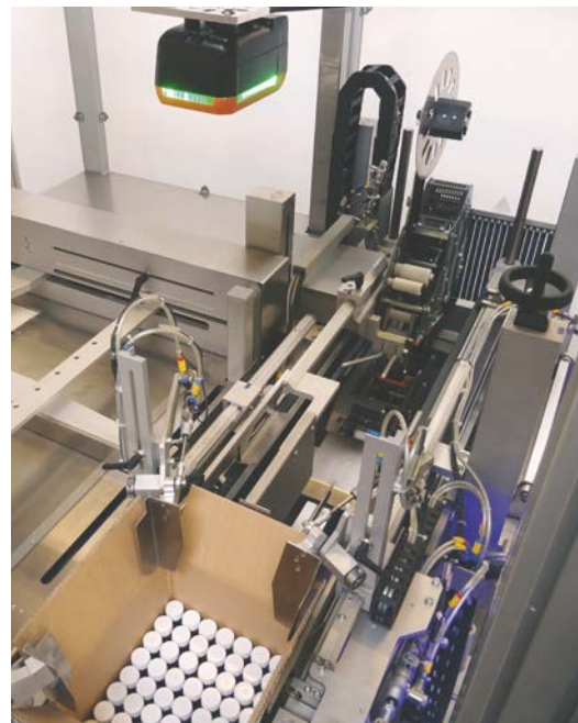
The CaseTeq machine from Christ is more flexible, manageable and user friendly thanks to integrated machine vision from B&R.
