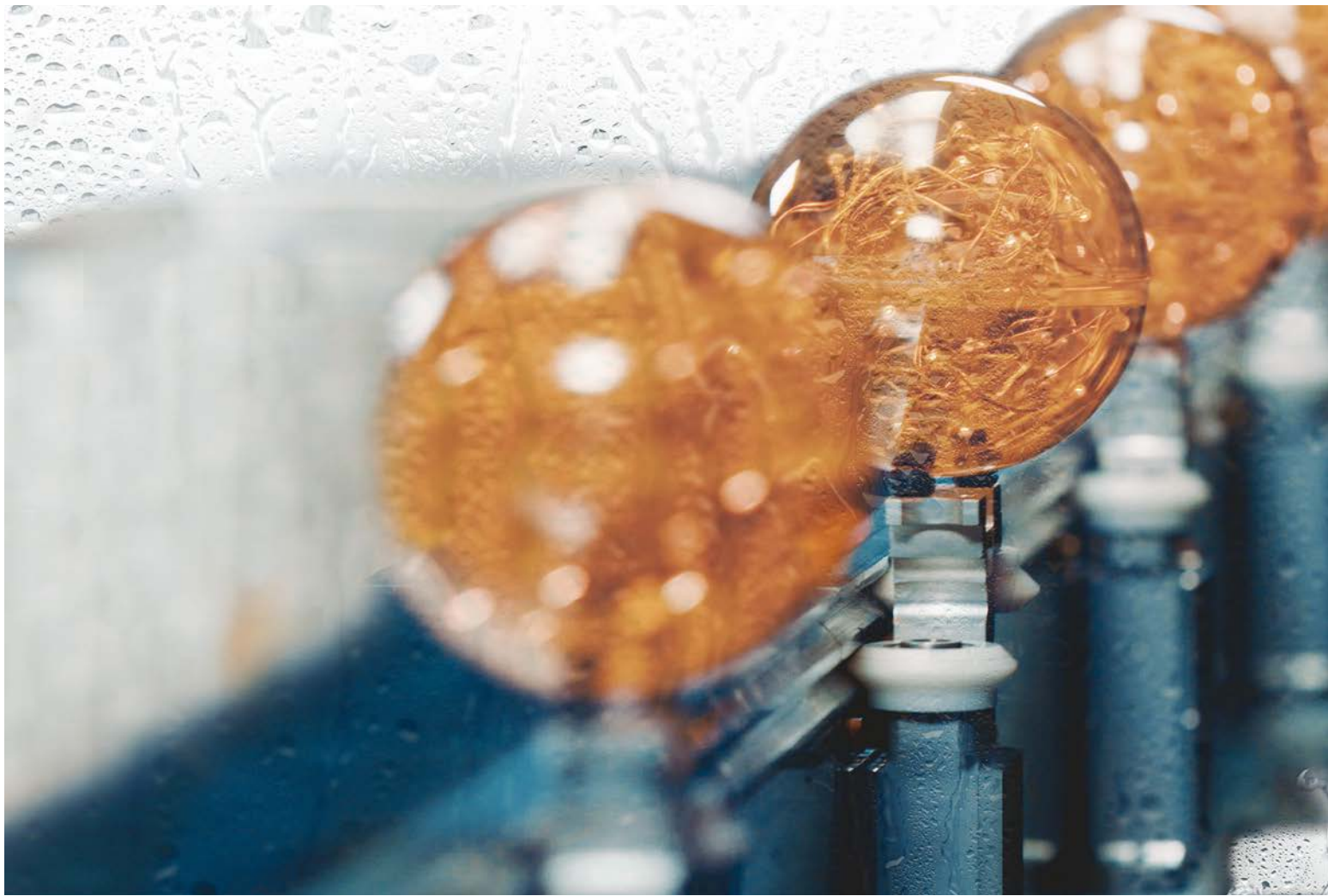
Completely enclosed stainless steel housing prevents even the tiniest ambient particulate matter from penetrating into the interior of the shuttles and track segments.
