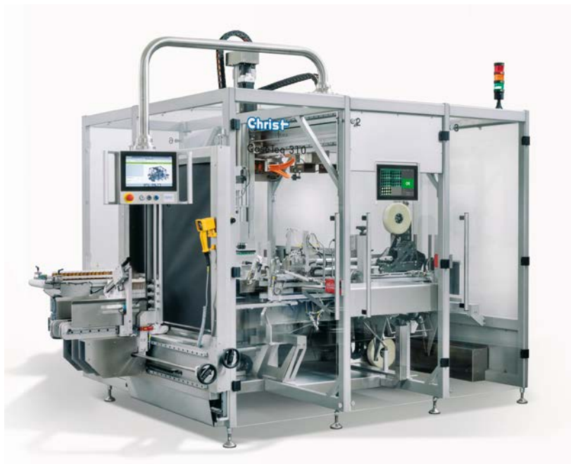
The CaseTeq case packer from Christ is a powerful, fully automatic horizontal system for erecting, packing and closing pre-glued shipping cases. Cameras from B&R will now be performing various inspection tasks.
