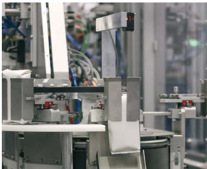
Thanks to SuperTrak's freely programmable movement profiles, designers have more freedom in how to arrange the processing stations, and can skip or add stations as necessary.
