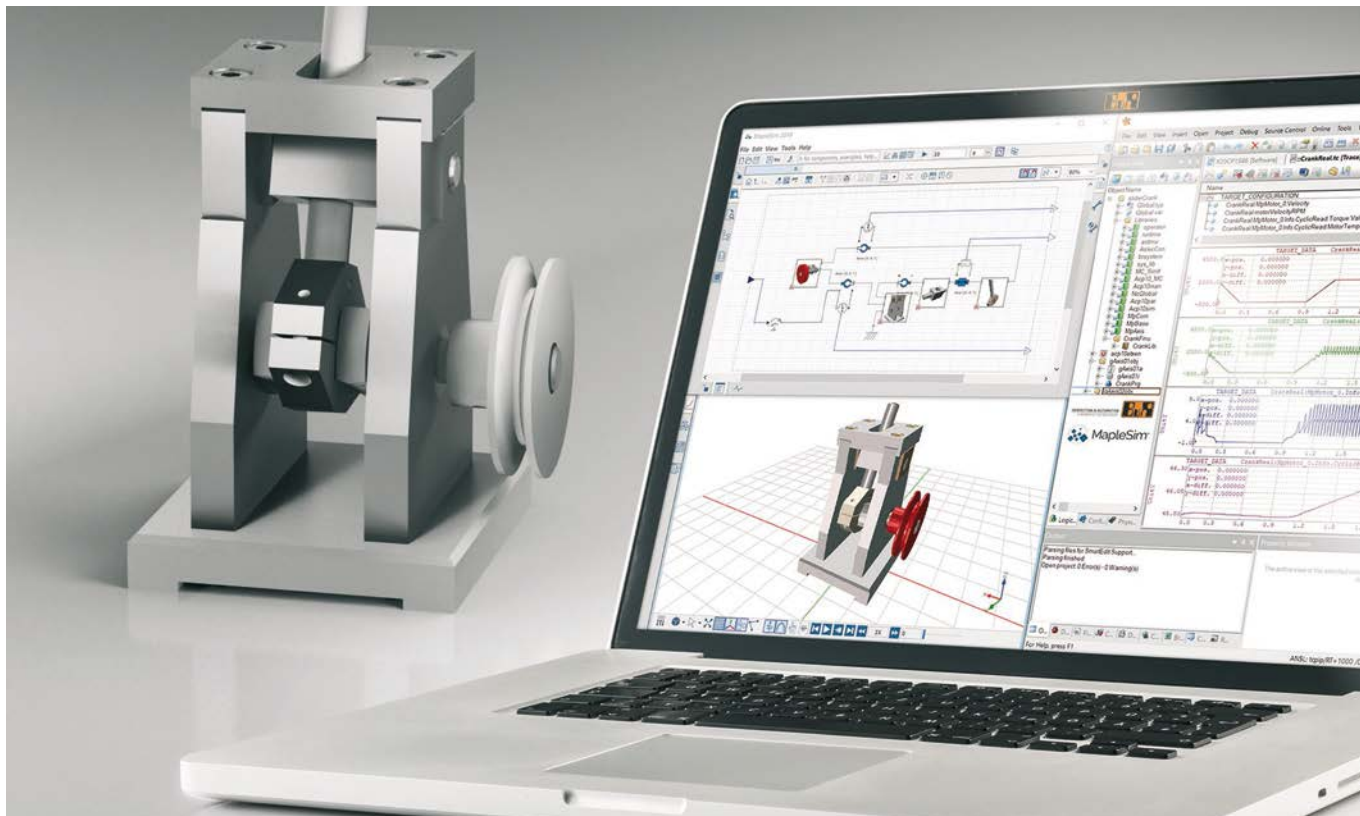
From MapleSim, they can export an FMU to transfer the model along with all the equations and CAD data to B&R's Automation Studio engineering environment.
