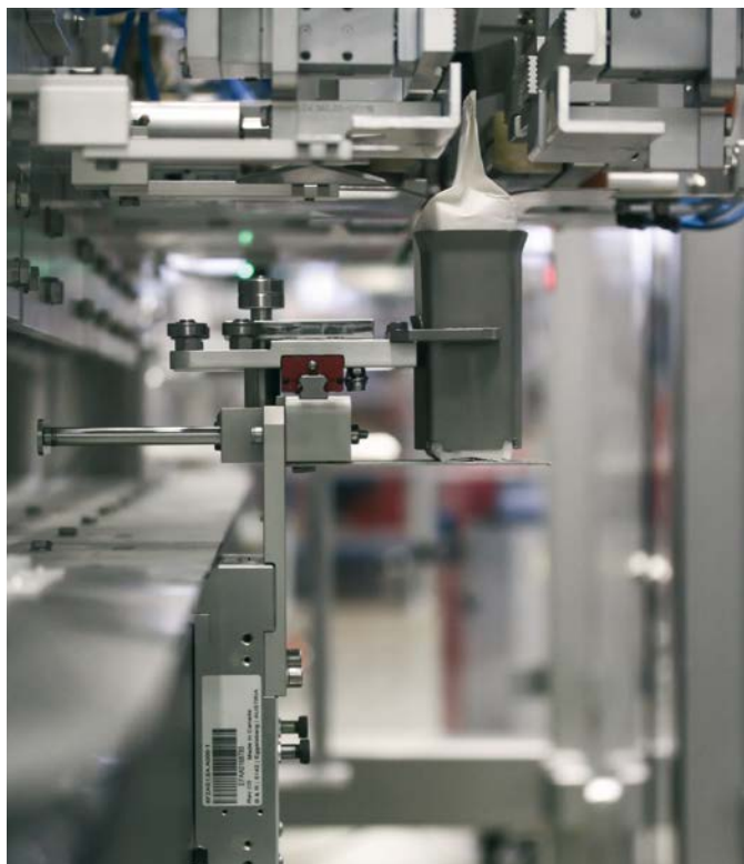
The transport system of the top closing machine moves each of the bags to the processing stations individually.
