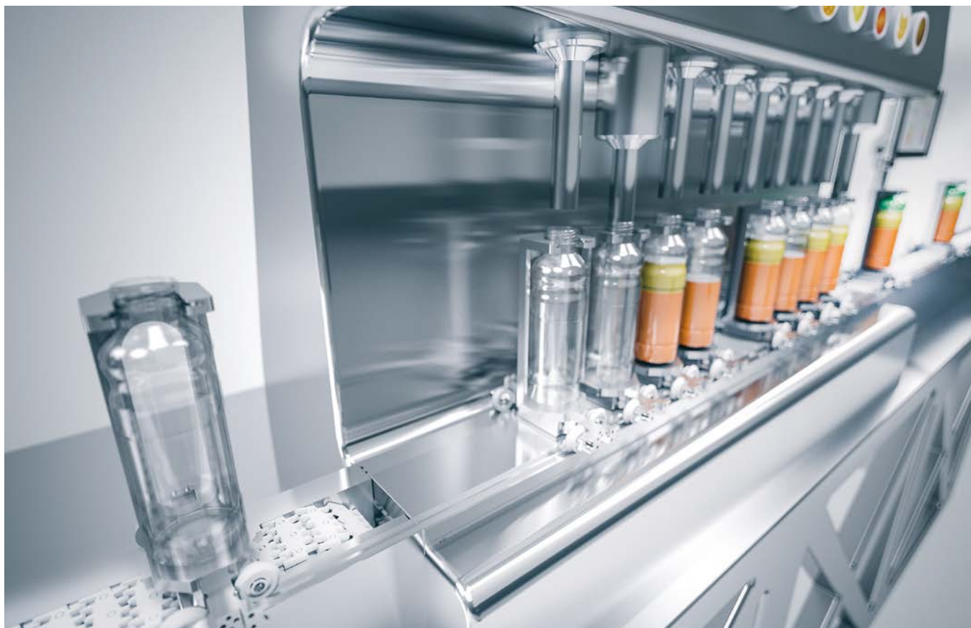
Guide rails ensure seamless transitions between the conventional conveyor belt and the intelligent ACOPStrak.
