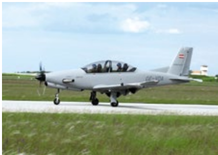
The DART-450 civilian aerobatic trainer has a maximum takeoff power of 500 horsepower, sidestick control and ejector seats.
