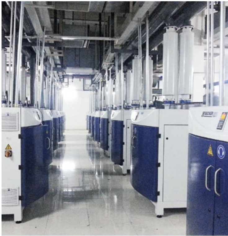
This central air supply system provides suction and blown air for multiple production lines in an energy-efficient way.
