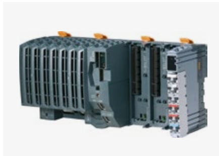
An X20 system with several CAN bus adapters and other interface modules was used in the rear of the research plane to record sensor signals.
