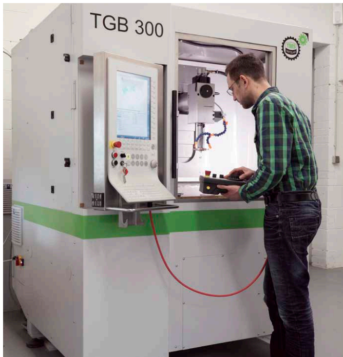
The TGB 300 glass machining center uses integrated safety technology from BSR with safely limited speed functions that allow the safety door to be kept open during setup.
