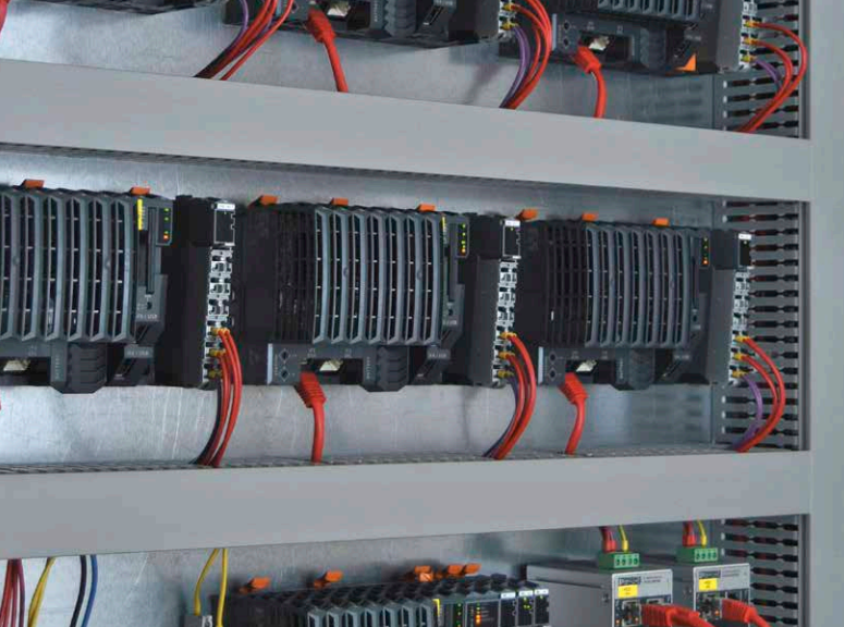
The redundant master computers in the central control room use a separate X20 I/O controller to communicate with each segment of the system.
