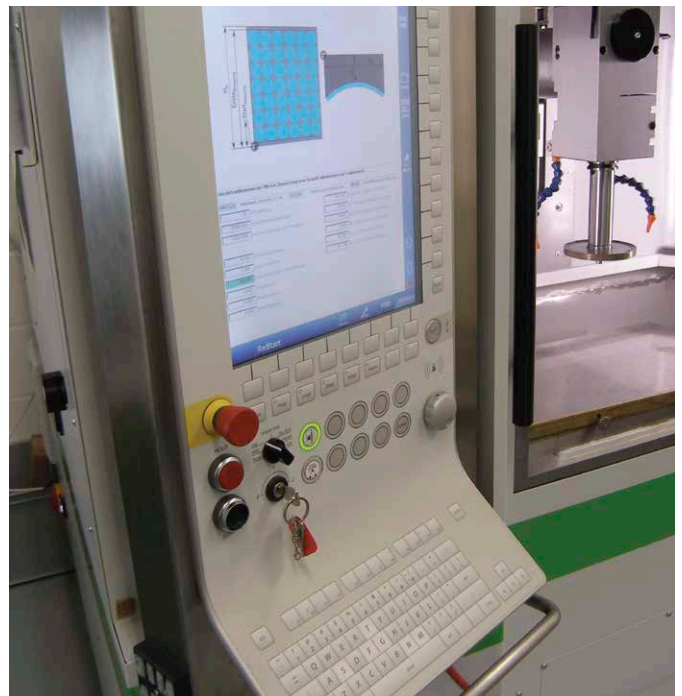
The CNC panel from BSR combines a touch screen display, key switch, keyboard and E-stop to provide all the control elements needed for a CNC machine in a single, ergonomic housing.
