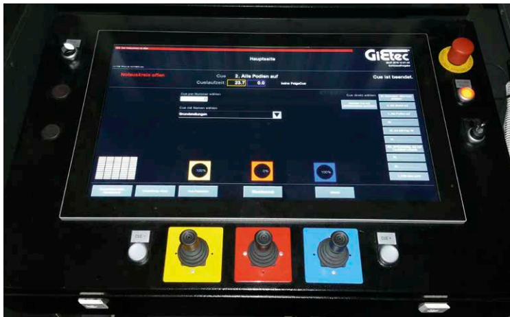
Two identical, multi-purpose Stage Controllers from Gietec, based on a Panel PC 900 with a projected capacitive 24" touch screen serve as control consoles for the 55 movable platforms that transform the stage during every performance of The Wyld .
