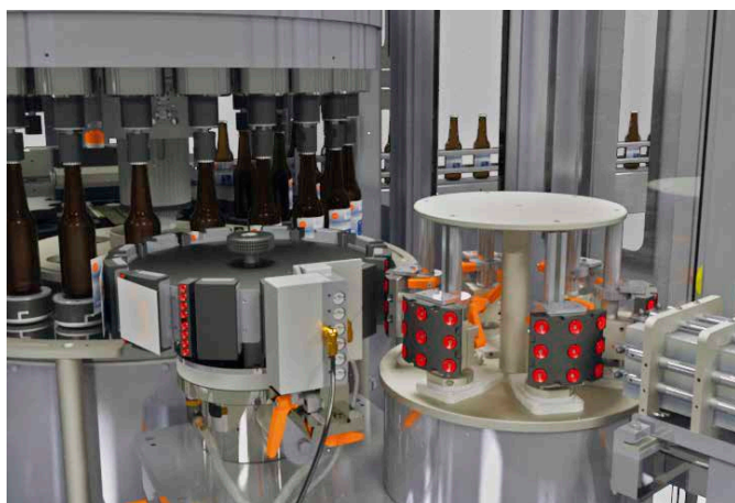
Driven by a B&R servo motor, the cut-and-stack module on the RL-840N labeling machine picks up labels, activates their adhesive and places them onto the containers.
