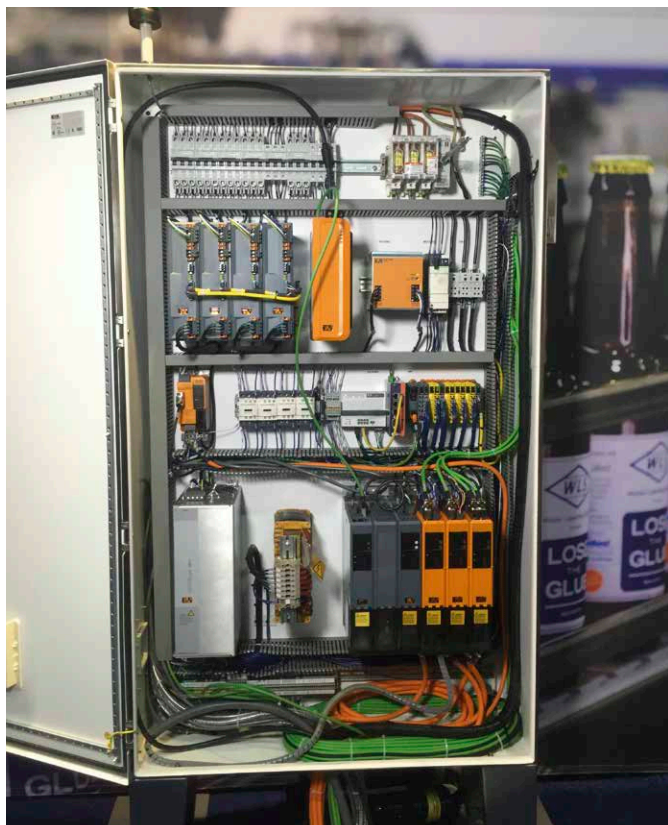
The RL-840N from WLS utilizes B&R control technology distributed throughout the machine – including ACOPDSmicro servo drives, ACOPDSmicro stepper drives, X20 and X67 I/O modules – to deliver a scalable and cost-competitive solution.
