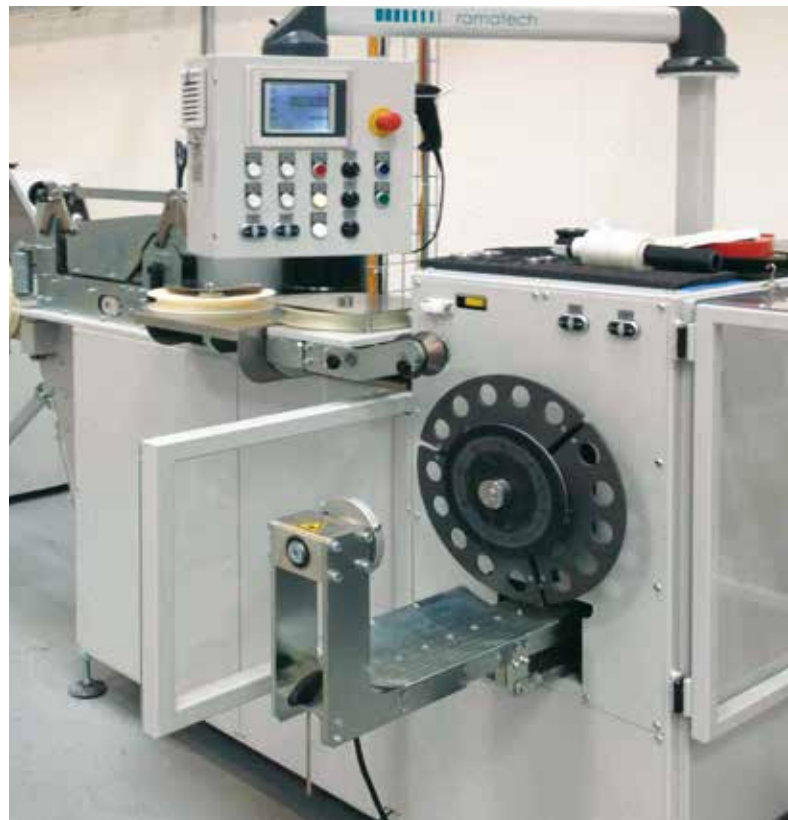
The layering unit and winding axis are controlled with precise synchronization. The optimized ergonomics of the operator console – featuring a B&R touch screen – ensure a clear overview at all times.
