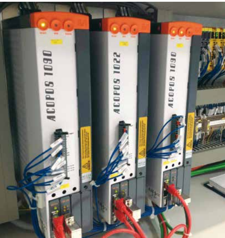
The speed and precision of B&R's servo drives allow the rewinder to achieve its certified speed of 3 meters per second.
