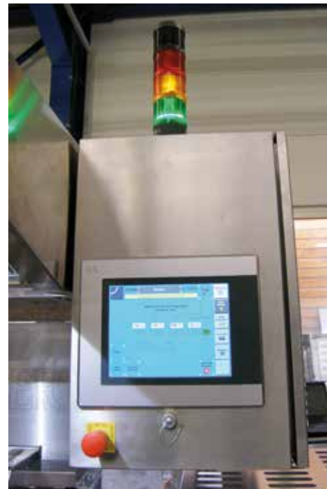
Opelka programmed the PLC and HMI applications entirely in B&R's Automation Studio engineering environment. The seamless integration made programming, diagnostics and maintenance remarkably efficient.
